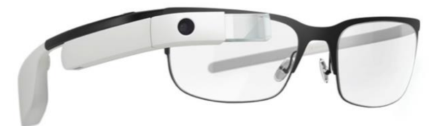
Google Glass: ~40 min recording per charge (nowhere near “always on”)
