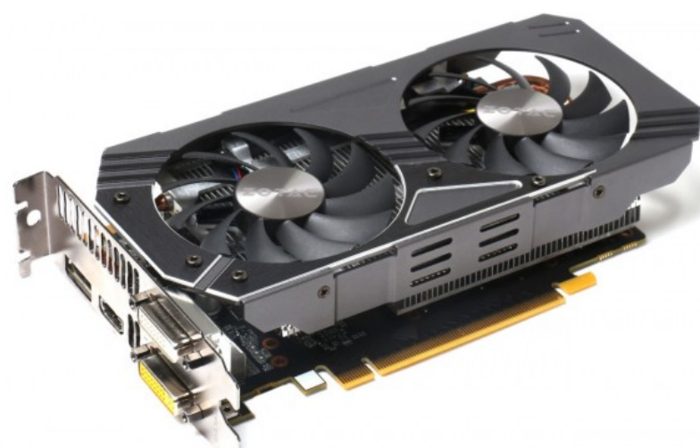
GTX 950: 6 SMM cores (90 watts)
